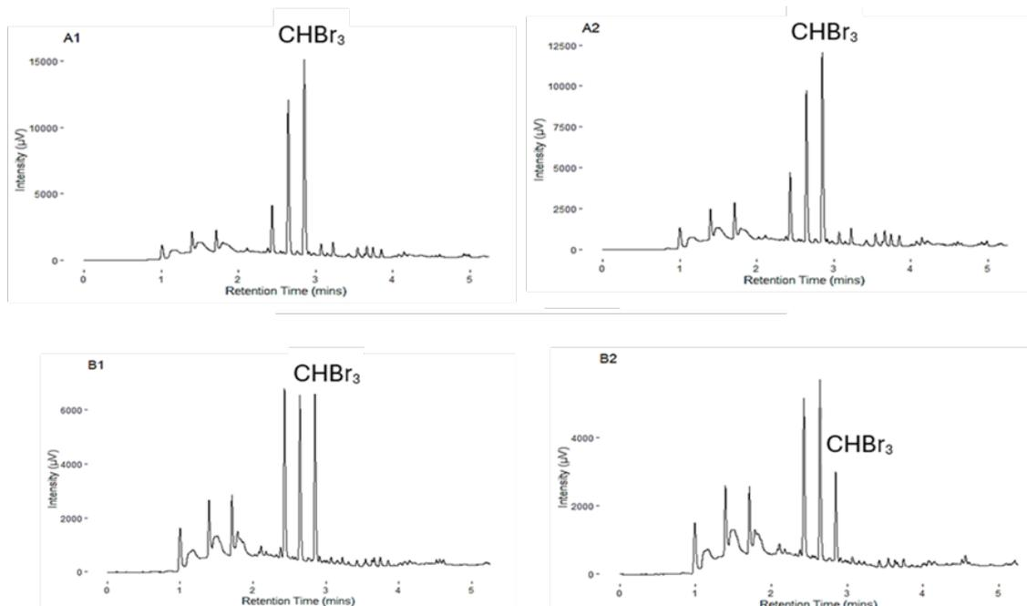
**Figure 5:** Chromatograms of Specimen A and B, illustrating the elution of bromoform with a retention time of 2.85 minutes.
